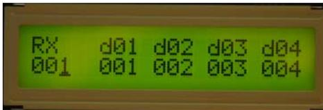
For any Active receiver, at any time, you can press and hold **the Select RX** button to display status information including the firmware version and current battery voltage. If no Active receiver is found, this is also reported.
