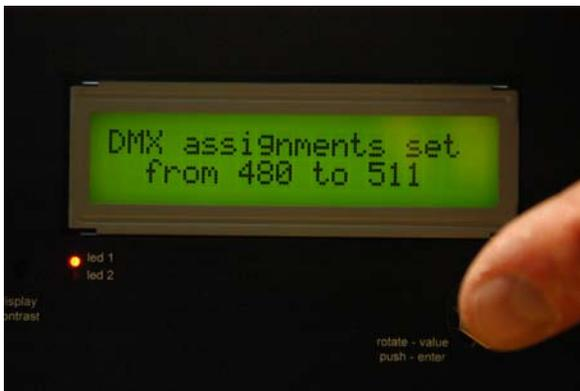
When first entering this mode, the DMX channel currently being watched is displayed as the starting channel. You may change this by turning the rotary control.
