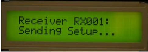
If the corresponding receiver is not Active, the transmitter LCD will report RXxxx Not Found. Otherwise, the LCD will report Setup Confirmed. The confirmation process verifies every parameter sent, while also retrieving the receiver firmware version, current battery voltage, and more.
