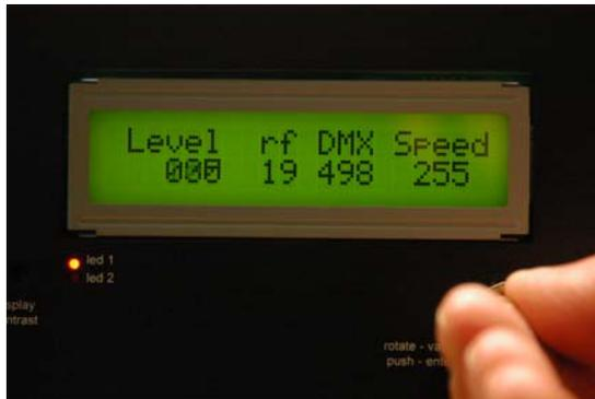
Select which channels will be part of the chase by pressing the **Manual Channel Test** key and making changes there. You can then return to the chase by pressing **Channel Chase Test**. It is not necessary to press **Exit** between these modes.
