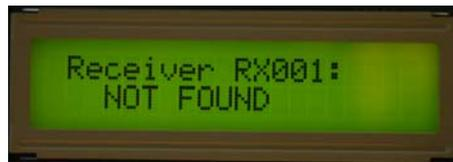
A radio-dimmer will assume a new RX number if it receives a control packet while the **Set RX** recessed button is held down. In this case, the RX value of that packet will become the new RX number for that receiver. Subsequent control packets for this RX number will be accepted and acknowledged with no need to hold down the Set RX button. (See the Receiver Operation section for additional information.)
