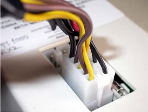
The RX4-STANDARD and RX4-HO (high output) receivers includes a 6-pin auxiliary power input connector:
