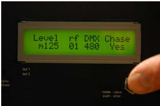
The Chase parameter is used by the Channel Chase Test function described below. It is toggled between Yes and No for the currently displayed rf channel by pressing the **Select/Enter** key.
