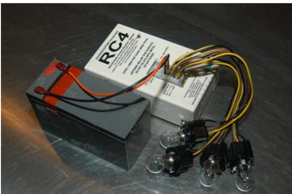
***Radio and dimmer control electronics will not operate properly with less than 10V of incoming power. This voltage must be maintained under load. Choose appropriately sized batteries and keep them charged.***
