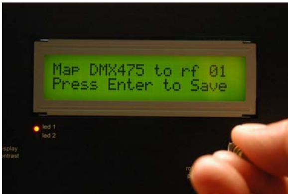
Similar to *Watch Channels* mode, the rotary control will select CV inputs above DMX 512 and below DMX 1. This makes it easy to assign any of the 8 available CV inputs to any rf dimmer channel, with the rotary control providing access to 520 sources (512 DMX channels and 8 CV channels).
