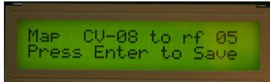
*HINT: Use the **Set DMX Start** function (detailed above) to create a map that is close to what you need. Then use the **Edit Assigns** key to add CV channels or otherwise adjust your channel assignments.*
