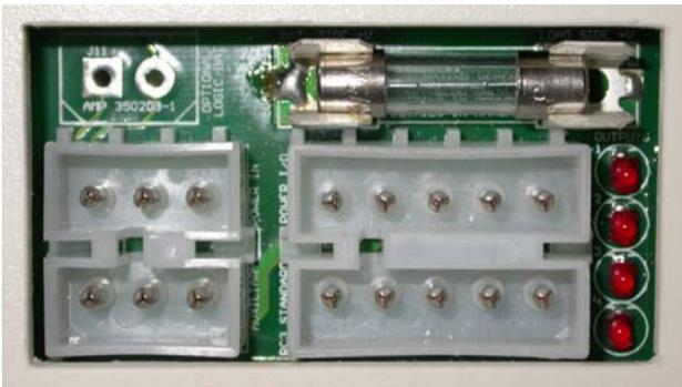
In some cases, the 6-pin connector can be used for high-power battery input, while the 10-pin connector can be used just for outputs. If all pins of both connectors are used, eight wires are available for both power in and dimmer out. This results in symmetrical current carrying capacity on both sides of the dimmers.
