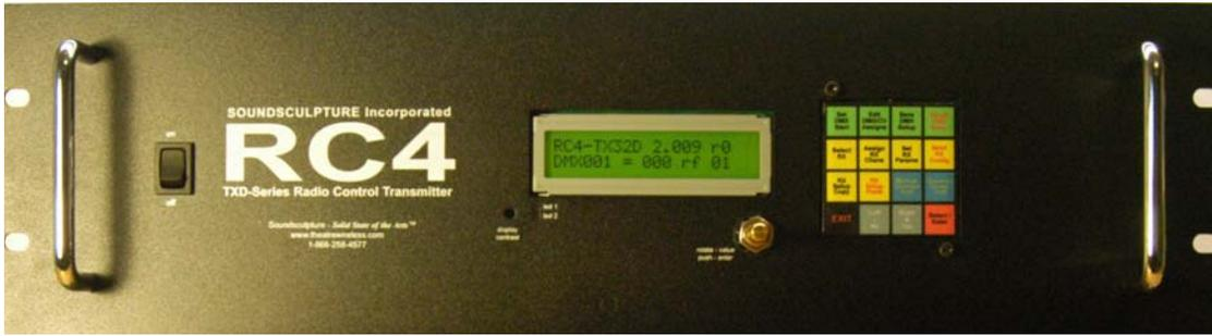
The TXD-Series radio transmitter user-interface consists of a 16-key keypad, a 20-character x 2-line LCD display, and a rotary control. The rotary control can also be pressed as a button, usually the equivalent of the **Select / Enter** key.
