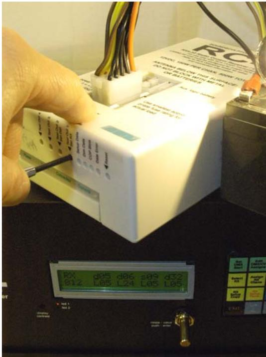
**NOTE:** *Some receivers may contain customized firmware for special applications. A specific RXnum is required to activate these custom processes. For example, a custom dual-motor speed control might be activated by using RX128. Customized receivers usually default to their special functions if defaults are loaded using the receiver's recessed buttons. Refer to the documentation supplied with your customized receiver for additional information about your specific unit.*
