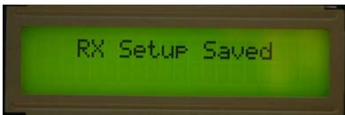
Similarly, the settings currently in scratchpad memory can be recalled to overwrite the currently displayed RX setup by pressing **RX Setup Paste**. All parameters are overwritten, including those not currently displayed.
