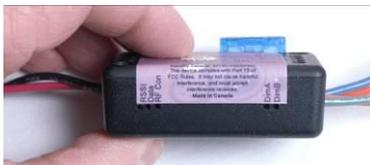
The **Data** indicator is on whenever data is being received by radio. *In normal operation this LED appears to blink rapidly, and will shimmer or flicker while DMX levels are changing.*
