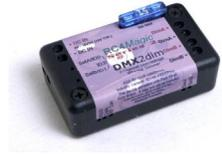
**MAXIMUM TOTAL OUTPUT POWER IS LIMITED BY CIRCUIT BOARD TRACE SIZE. User changeable Bussmann ATC load fuse should not exceed 15A and should be fast-blow type.**
