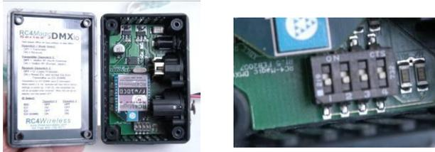
*Make changes with the power removed. New settings do not take effect until the next power-up.*
