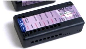
**MAXIMUM TOTAL OUTPUT POWER IS LIMITED BY CIRCUIT BOARD TRACE SIZE. User changeable Bussmann ATC load fuse should not exceed 15A and should be fast-blow type.**
