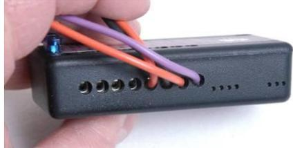
The **Data** indicator is on whenever data is being received by radio. *In normal operation this LED appears to blink rapidly, and will shimmer or flicker while DMX levels are changing.*
