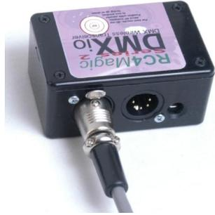
The DMXio receiver output is compliant with USITT DMX512/1990, and closely mimics the data going into the associated DMXio transmitter. It will output the same number of channels and the same timing between packets. DMX packets can contain anywhere from 1 to 512 channels, with a frame rate of anywhere from 12 packets to thousands of packets per second. (Of course, high frame rates require fewer channels in each packet.)
